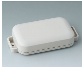
C3206107 EASYTEC 100 ASA+PC (UL 94 V-0) off-white RAL 9002 4.76"x2.44"x1.02" IP 65 opt., IP 40
