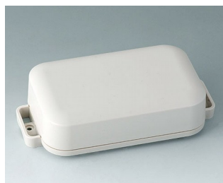
C3207207 EASYTEC 125 ASA+PC (UL 94 V-0) off-white RAL 9002 5.79"x3.07"x1.46" IP 65 opt., IP 40
