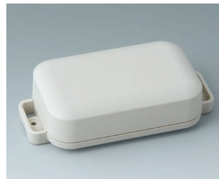
C3206207 EASYTEC 100 ASA+PC (UL 94 V-0) off-white RAL 9002 4.76"x2.44"x1.22" IP 65 opt., IP 40
